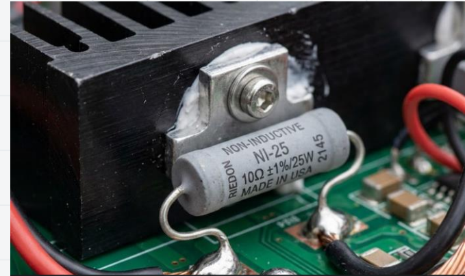
FIG 1.0: NON-INDUCTIVE HEATSINK RESISTOR ASSEMBLY
