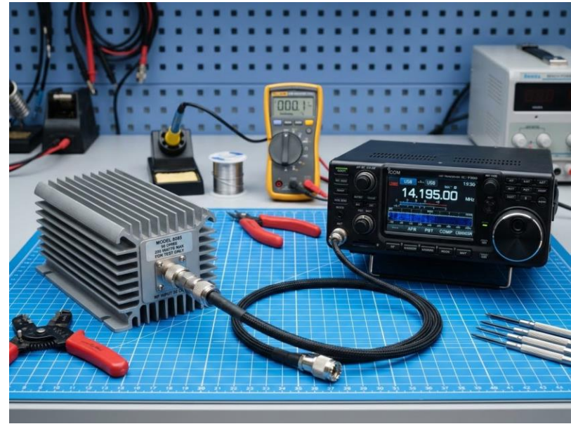
FIG 1.1: 50-OHM DUMMY LOAD CONNECTED TO TRANSCEIVER TEST BENCH
